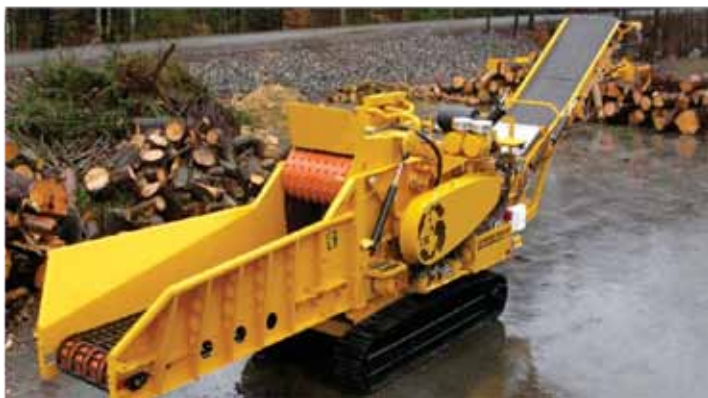
THE MAGNUM FORCE 5400 CAT C18 765 HP ENGINE
