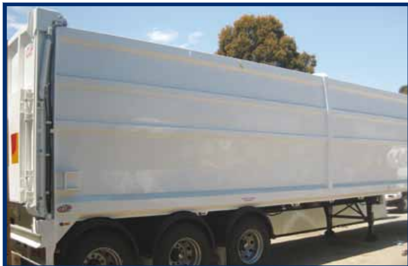
The new style of rear ejection waste trailer, BTE's GENESIS.
