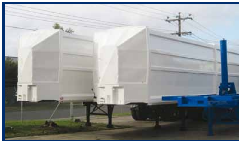
The body design of the new GENESIS addresses some OH&S issues with many of the old ejection trailers.
