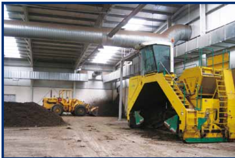
Windrow turner in the aerobic hall – compost plant.
