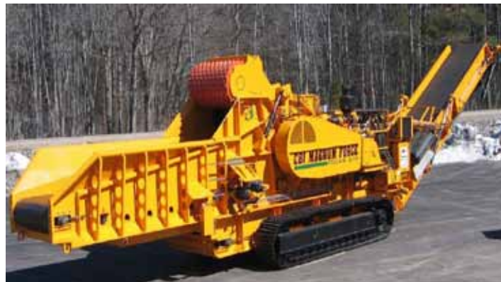
THE MAGNUM FORCE 6400 CAT C32 1150 HP ENGINE
