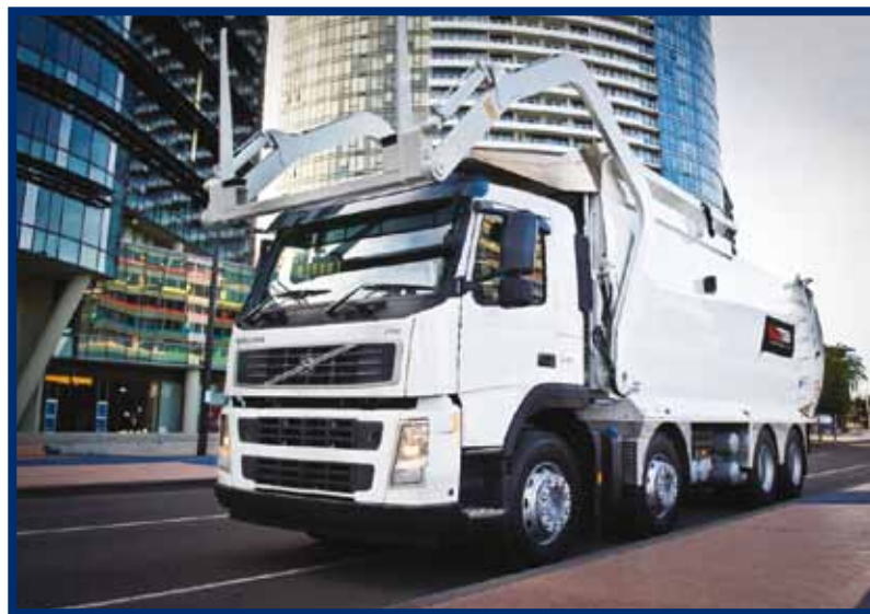
The introduction of Hardox has brought a dramatic change in wear and working life of front lifts
